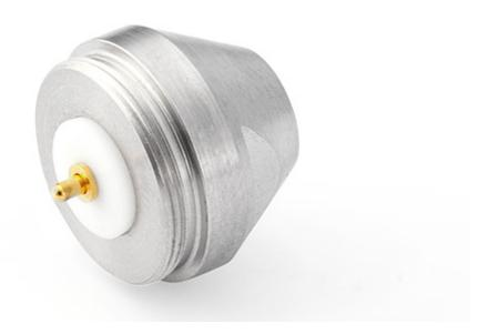
Length: 10 mm Inner threading for preamp.: 5.70-60 UNS-2 Outer threading for mic.: 11.70-60 UNS-2 Material: stainless steel
