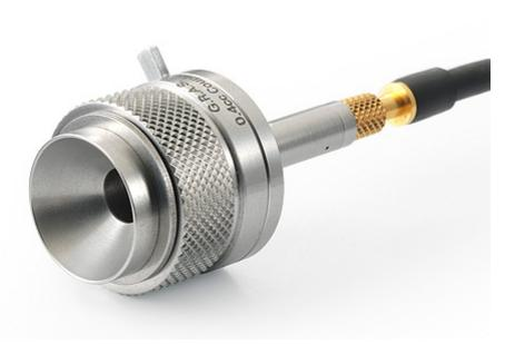
Connection: CCP Volume: 0.4cc IEC: 60318-8 Use: For hearing aid test up to 16 kHz Special Feature: <25 dB(A) noise floor
