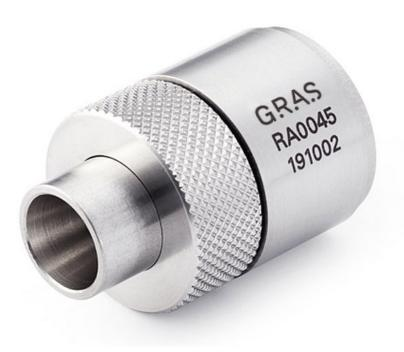
Standards: IEC 60318-4 (based on), ITU-T P.57 Eff vol: 1260 mm<sup>3</sup> @ 500 Hz Res freq: 13.5 kHz ±1 kHz The GRAS RA0045-S4 Ear Simulator is an ear simulator with an acoustic input impedance closely resembling that of an average human ear. The RA0045-S4 includes a 40AP pressure microphone and each RA0045-S4 is individually calibrated with this specific microphone.
