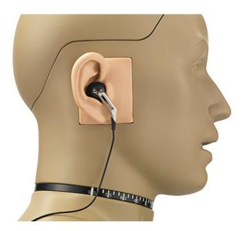
Connection: Traditional Power Supply (200 V/LEMO) Channel(s): 1 ANSI: S3.36 Based on IEC 60318-7 Based on ITU-T Rec. P.58 The 45BB-11 KEMAR is an acoustic research tool with a built-in low-noise ear simulator for testing of ear and headphones and in-ear ear protectors with or without active noise cancellation. Its corresponding two-channel equivalent is <u>GRAS 45BB-12 KEMAR with</u> <u>Anthropometric Pinnae for Ear- and Headphone Test, 2-Ch LEMO.</u>
