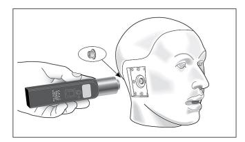
In most cases calibration can be done from the outside without dismantling the ear simulator(s).
