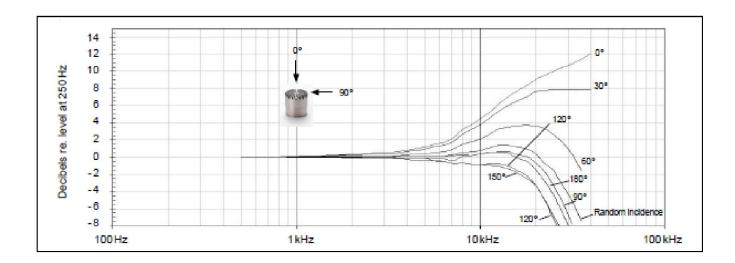
Free-field corrections for various degrees of incidence
