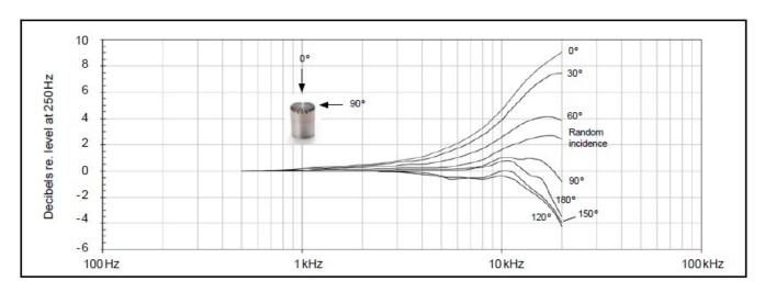
Free-field corrections for different angles of incidence
