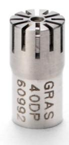
Freq range: 6.5 Hz to 140 kHz Dyn range: 49 dB(A) to 178 dB Sensitivity: 1 mV/Pa The 40DP is an IEC 61094 ½ externally polarized pressure microphone with rear-venting. Due to its tiny size, this high-precision condenser microphone can be used to measure very high-frequency sounds without disturbing the sound field.
