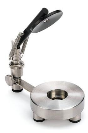
For use with GRAS couplers and artificial ears. It has an adjustable spring-loaded arm to exert a variable force on the test object.
