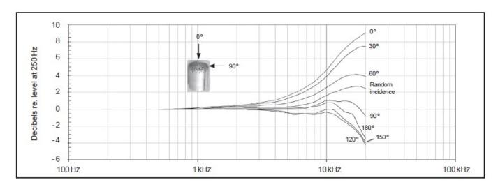
Free-field corrections for different angles of incidence
