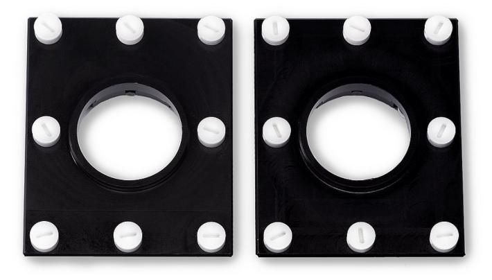
Kit with plastic ear holder plates and plastic ear canal extensions. For test of binaural hearing aids which are based on radio frequencies.
