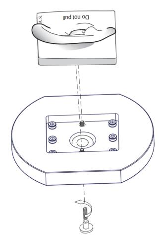
GRAS anthropometric pinna mounted on a 711-style (IEC 60318-4) ear simulator using the RA0517 kit
