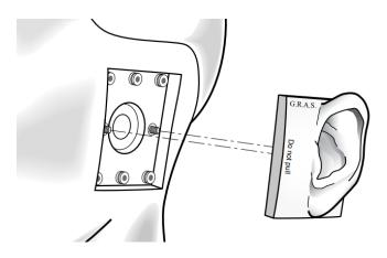
The external shape of the pinna is identical to that of the standardized KEMAR pinna, but concha and canal have been modified so that they closely mimic the properties of a real human ear. The ear canal has been extended and is an integral part of the pinna that now seals directly against the ear simulator. Like the human ear, the ear canal now has the 1st and 2nd bend, and the interface with the concha is oval.
