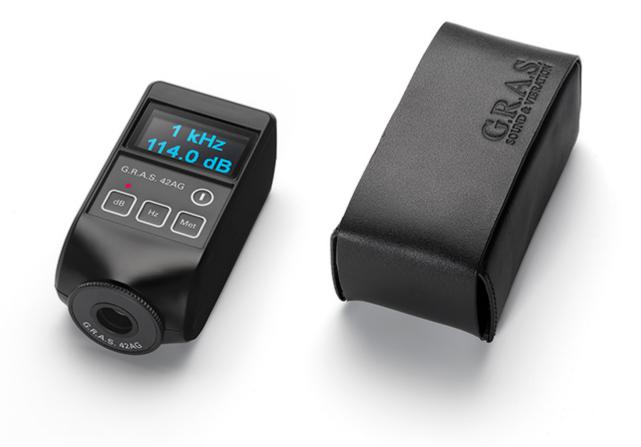
Sound pressure level: 94 dB or 114 dB Frequency: 250 Hz or 1 kHz ANSI: S1.40 IEC: 60942 class 1 The GRAS 42AG Multifunction Sound Calibrator is a portable, battery-operated precision microphone calibrator. The calibrator can be used directly on 1" microphones. Adapters for calibrating 1/2" (factory mounted), 1/4" and 1/8" microphones are included.
