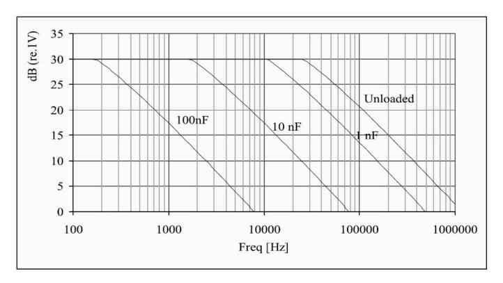
Typical max. rms output signal with 120 V and 30 V supply
