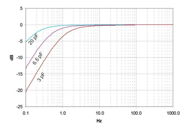
Typical low-frequency response of Type 26AL for  $\frac{1}{2}$  (20 pF),  $\frac{1}{4}$  (6.5 pF) and  $\frac{1}{6}$  (3 pF) microphones
