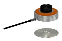
When the 147AX microphone set is placed over the mounting disc, a center guide ensures that the microphone will be attached and centered to the disc correctly once the magnetic force kicks in. In this way, it is easy to mount in difficult-to-access locations with no loss of placement accuracy.
