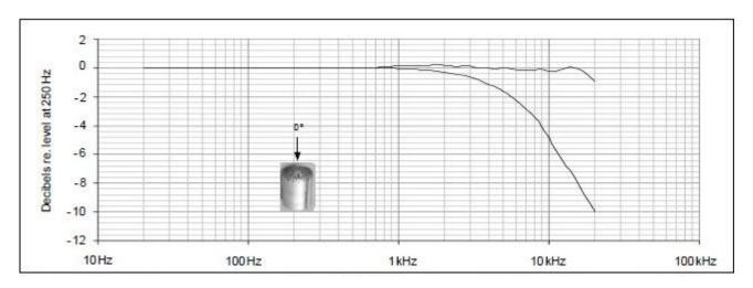
Typical frequency response. Upper curve shows free-field response for 0°, lower curve shows pressure response.
