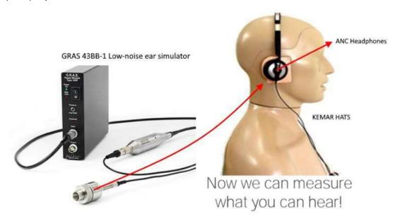
Figure 1. GRAS 43BB-1 Low-noise ear simulator can be mounted inside a KEMAR HATS for low-noise measurements down to 10.5 dBA.
