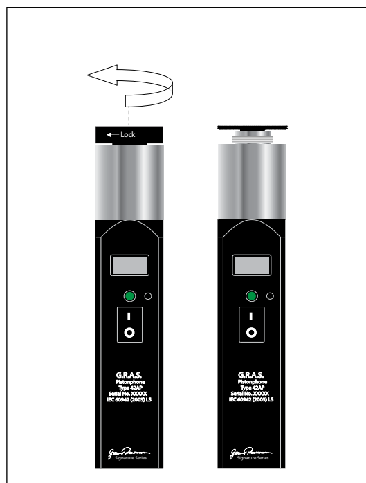
Fig. 20. Loosening or removing the Collar Ring.
