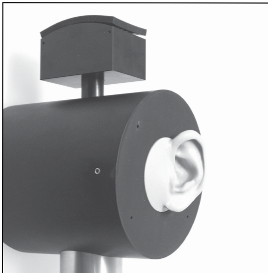
Fig. 4. Mounting the KEMAR pinnae
