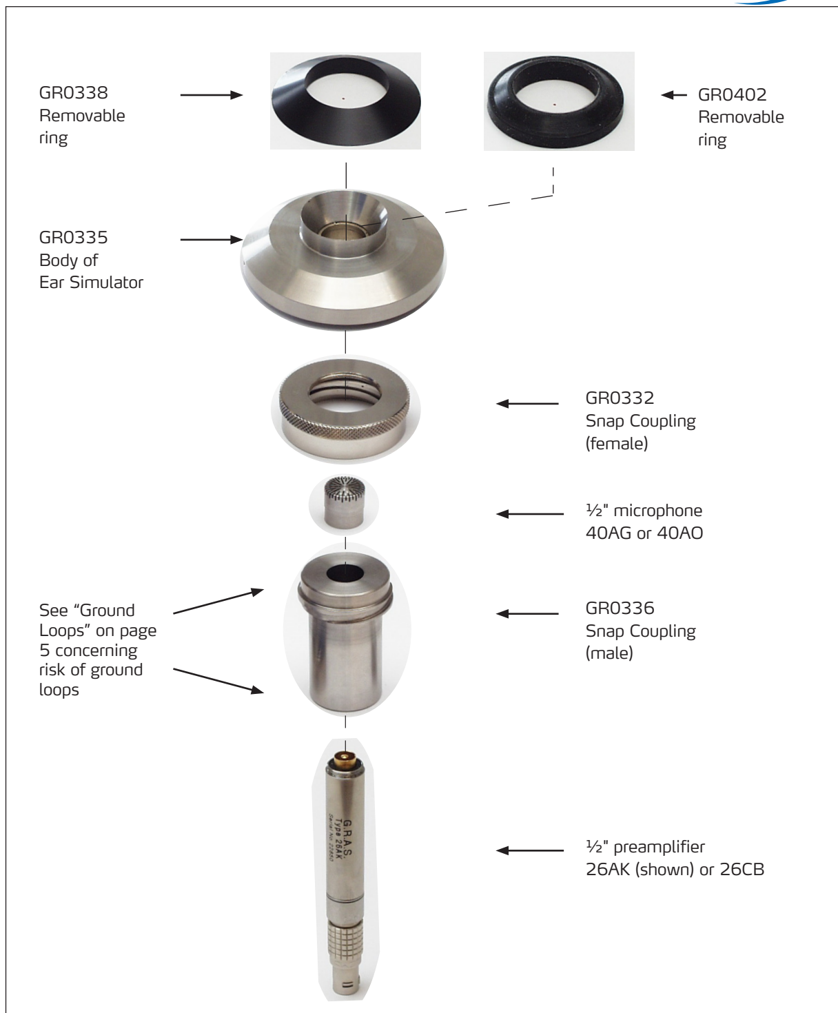
Fig. 7. Exploded view of all the user-serviceable components of the 43AD (mounting plates and extension cable omitted for clarity)
