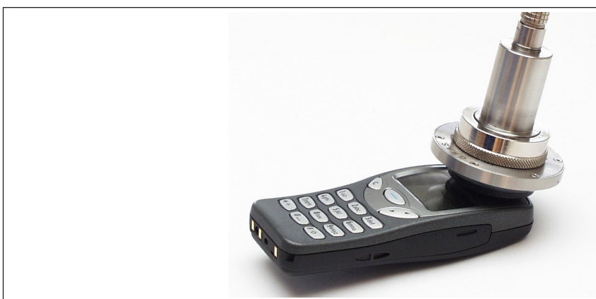
Fig. 6. Place the Ear Simulator centrally over the earpiece of the mobile phone
