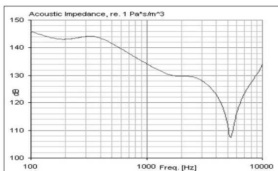
Fig. 11. RA0039 acoustic input impedance
