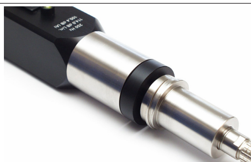
Fig. 5. Gently push the microphone into the Pistonphone's coupler until it reaches the stop
