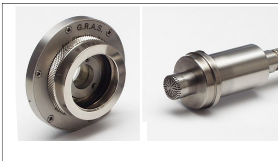
Fig. 4. Showing the two halves of the snap coupling to give quick access to the microphone
