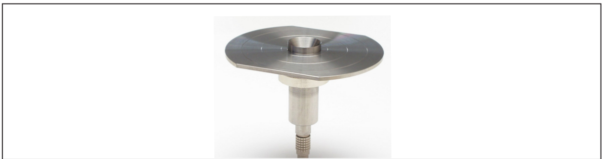
Fig. 2. 43AD shown with mounting plate GR0339 for testing earphones fitted with fluid cushions (circum-aural)
