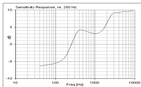
Fig. 12. RA0039 closed-coupler frequency response
