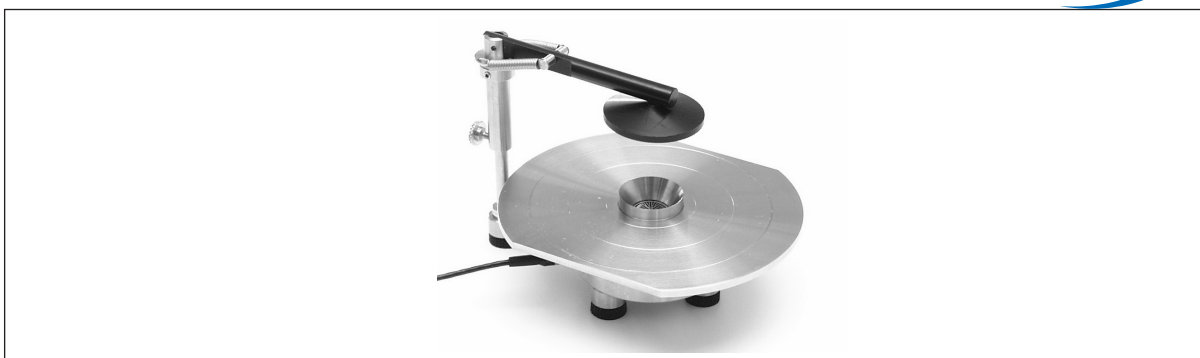
Fig. 2. 43AA shown with mounting plate GR0339 for testing circumaural earphones
