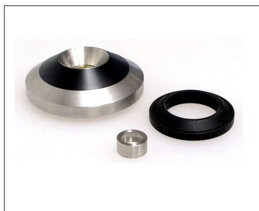
Fig. 9. RA0039 Ear Simulator as delivered
