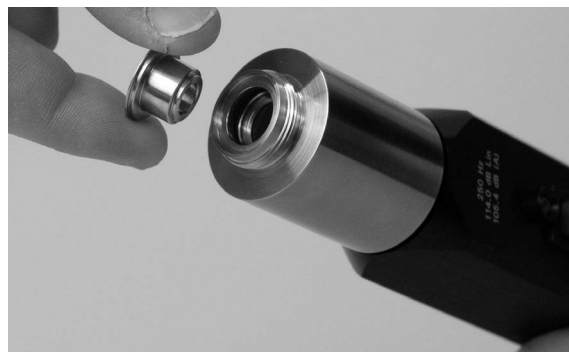
Fig. 18. Mount the adapter RA0157 on the pistonphone.
