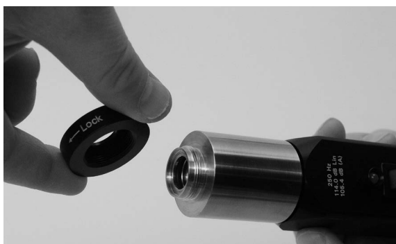
Fig. 17. Loosen the retention collar on the pistonphone.
