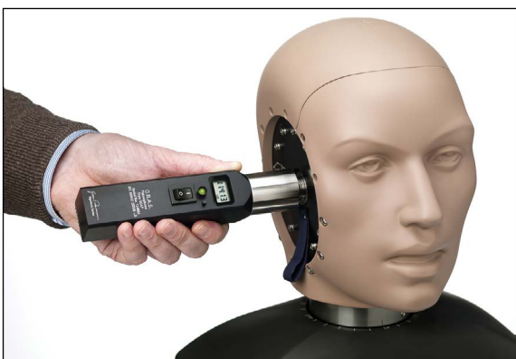
Fig. 19. Place the pistonphone onto the ear canal.
