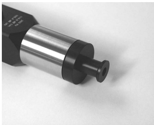
Fig. 3.4 1/4" microphone adapter inserted in the coupler
