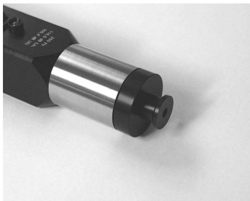
Fig. 3.5 1/8" microphone adapter inserted in the coupler
