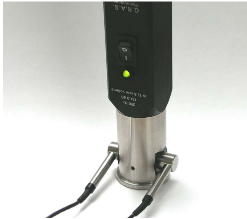
Fig. 4.1 Two-port Coupler RA0042 shown here with the two phase-matched microphones of an intensity probe
