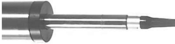
Fig. 3.3 1/2" microphone inserted in the coupler
