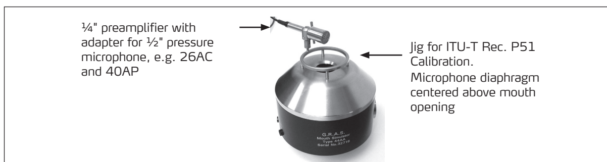
Fig. 8. Set-up for calibrating the Mouth Simulator according to ITU-T Rec. P51
