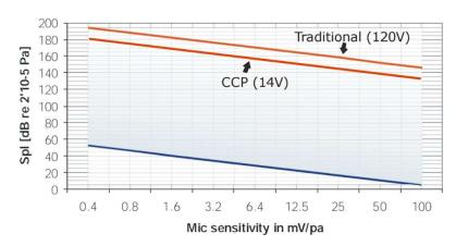
Figure 4. Comparison of upper dynamic range limits of the same microphone using a CCP vs Traditional preamplifier.
