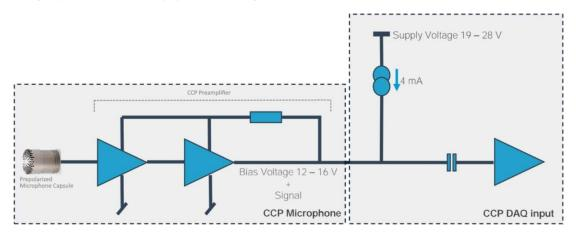
Figure 2. CCP microphone set connection layout including Prepolarized microphone capsule, preamplifier and DAQ input with built in CCP supply.
