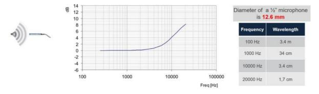
Figure 4. Pressure build-up for a ½" pressure microphone pointing at 0-degree incidence from sound source in a free-field environment.
