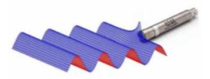
Figure 3. ½" pressure microphone set exposed to high frequency sound wave with short wavelength. Diffraction effect appears.
