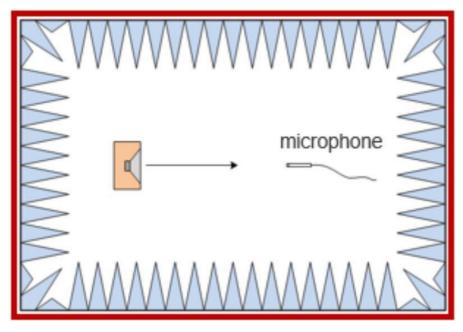
*Figure 1. Pressure measurement microphone pointed at 0-degree incidence from a sound source inside an anechoic chamber (Free-field environment).*
