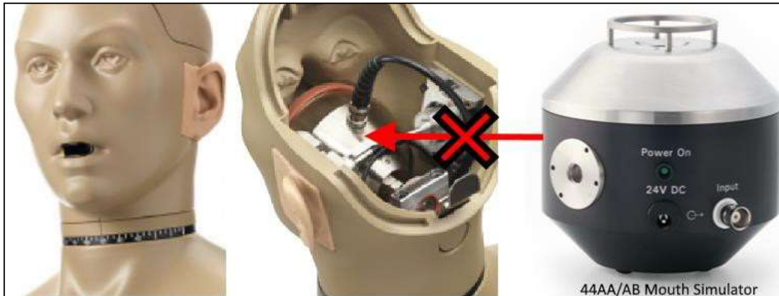
Figure 1. 44AA/AB mouth simulator CAN'T fit inside a GRAS 45BC KEMAR's head.
