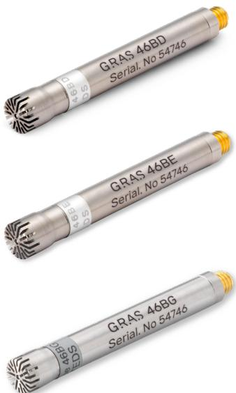
while maintaining reliable sensitivity. Such pressure mics are ideal for measuring sound pressure at boundaries (or “at the wall of the pressure wave”) and are commonly used when a strong, overpressure event must be recorded without clipping.
