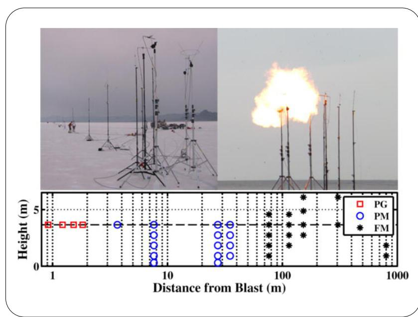
Picture from the publication. "(Color online) View of the microphone array on the Bonneville Salt Flats, a balloon explosion, and a schematic of piezoresistive gage (PG), pressure microphone (PM), and free-field microphone (FM) locations."
