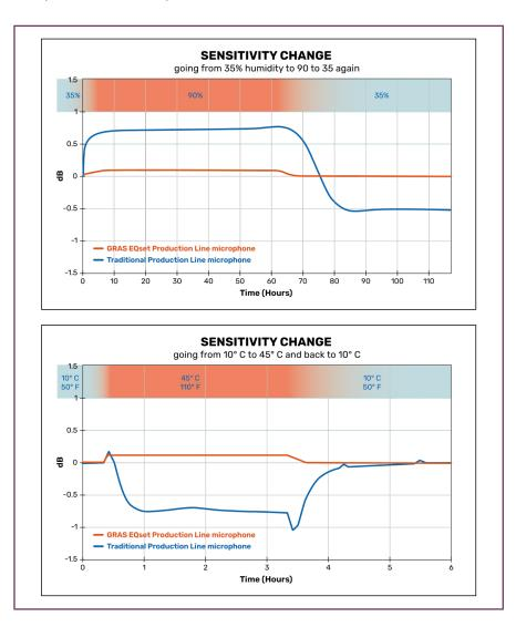
Yet another benefit of microphones with EQset technology is their higher environmental stability as compared to other production line microphones. EQset microphones produce the same precision measurements regardless of the climate your production lines operate in, using the same test equipment across the board and requiring far less validation and adjustment.
