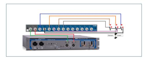
FIGURE 11. Setup with APx517.
