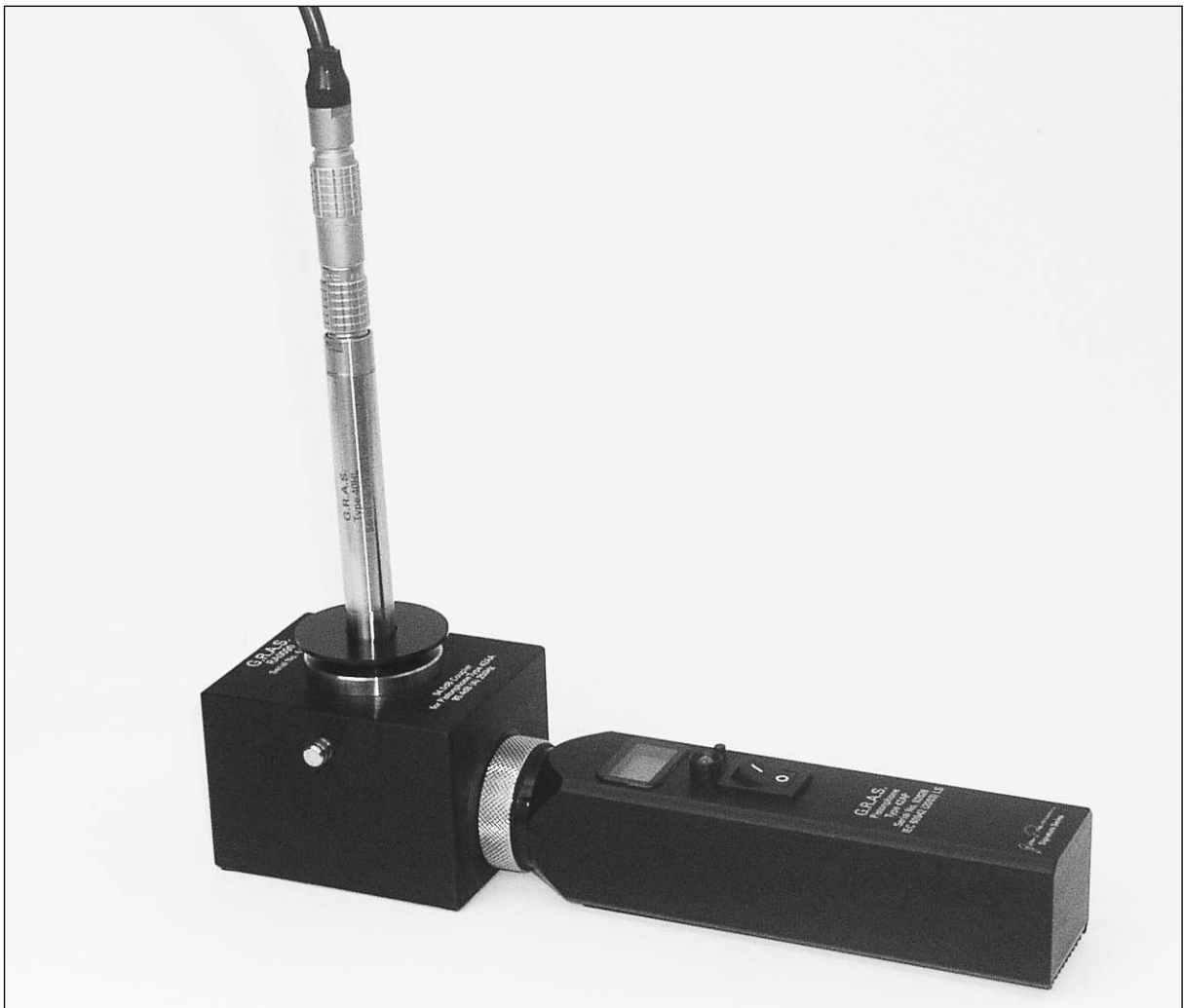
Fig 2.2 Pistonphone fitted with Coupler RA0090 and the microphone inserted into the coupler. The spring arrangement supplied with the coupler is not used.
