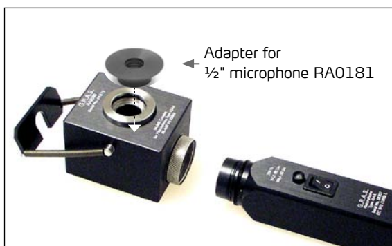
Fig 2.1 Pistonphone without its normal coupler and ready to accept the Coupler RA0090
