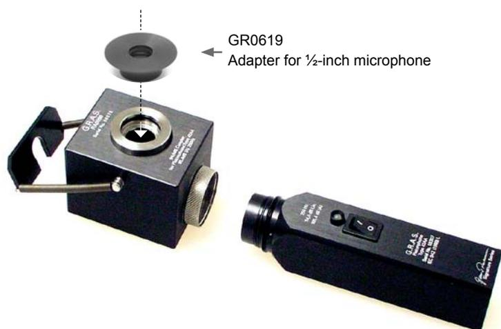
Fig. 3.1 Pistonphone without its normal coupler and ready to accept the Coupler RA0090
