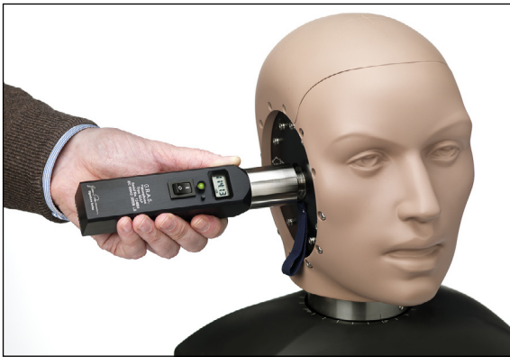
Fig. 17. Place the pistonphone onto the ear canal.
