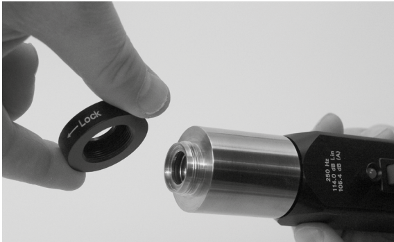
Fig. 15. Loosen the retention collar on the pistonphone.
