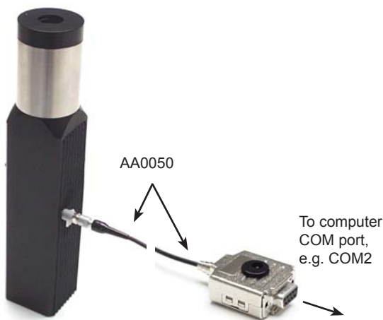
Fig. 2 Pistonphone connection for use with a computer
