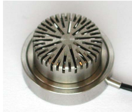
Fig. 1 An unmounted 47AX-S1, the microphone used in the 67AX.
