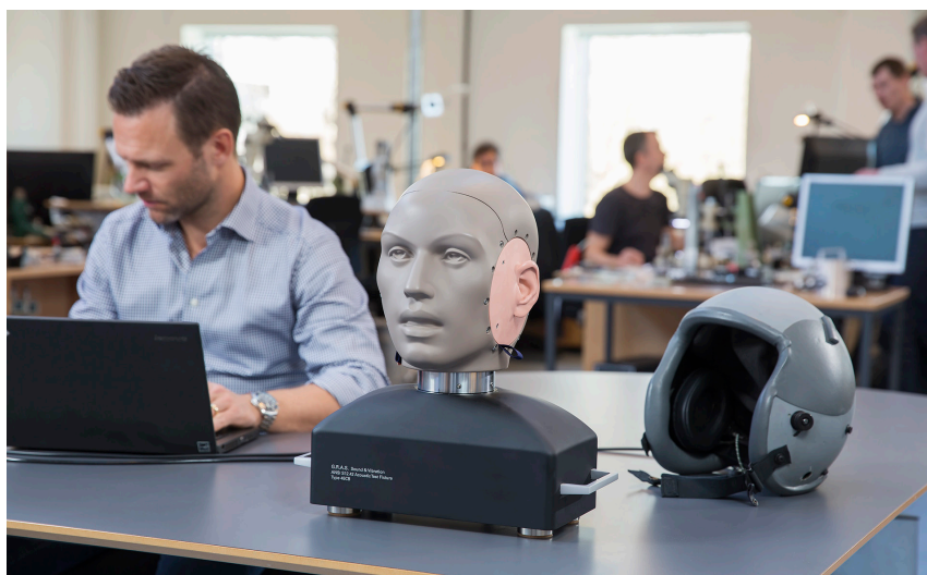
The GRAS 45CB, also called the ANSI-head because it meets the American ANSI-ANSA S12.42 Standard.
