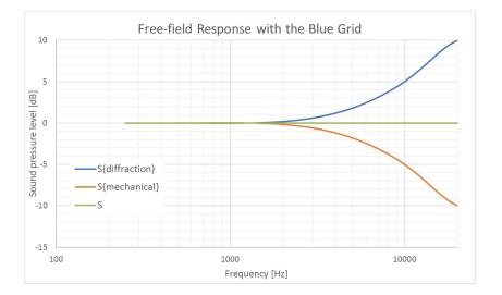
Figure 1 Free field response of 146AE with the Blue Grid
