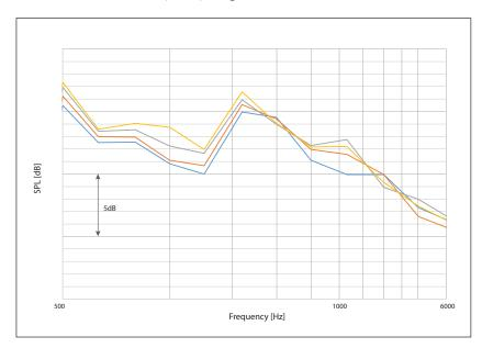
One of many conclusions from the initial method investigation was that the precise transducer mounting position and orientation was extremely critical in order to obtain repeatability. Also, differences in operator interpretation of the positioning instructions could generate differences in the results.
