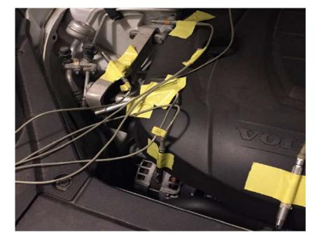
Figure 4 Microphones mounted in the engine bay
