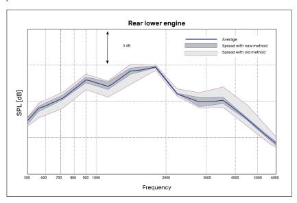
Figure 13 Repeatability for three points near rear engine, with old and new method
