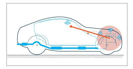
Figure 1 Acoustical transfer from engine bay
