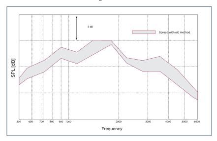
The new method shows variation within 0.2 dB in the same frequency range, even with only 13 microphones as opposed to the 24 microphones for the old method, as shown in Figure 12.
