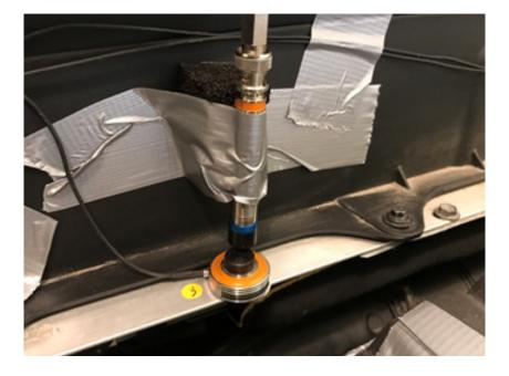
Figure 4 Pressure and free-field microphone mounted facing each other
