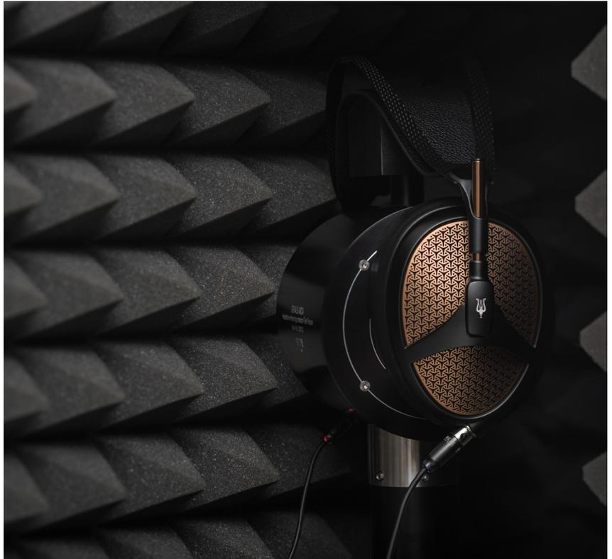
*"The anthropometric pinna enables us to improve the sealing of our headphones, providing us with repeatable and consistent measurements"* Mircea Fanatan elaborates. For Meze Audio, the combined advantage of the 45CA, the anthropometric pinna and the High-frequency Ear Simulator is better test results in the audible range and a significant improved sealing on their headphones.
