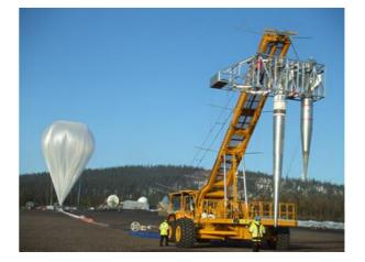
Figure 10: N-WAVE and Low-Boom Models being prepared for drop.
