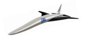
Figure 12: Experimental supersonic airplane model (unmanned aircraft with no engine and capable of autonomous flight) to be used in D-SEND#2.
