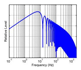
Figure 1: Acoustic content of a sonic boom.
