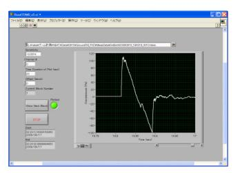
Figure 5: Instrumentation graphical user interface of outdoor recorded sonic boom.
