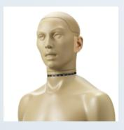
Improved materials KEMAR's previous fiber glass construction has been updated to a plastic composite that provides a more user friendly and ruggedized construction
