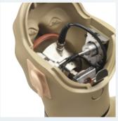
Snap fit ear simulators Mount and dismantle the ear simulators with one hand for ear-canal exchange or calibration
