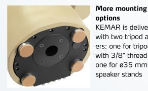
options KEMAR is delivered with two tripod adapters; one for tripods with 3/8" thread and one for ø35 mm loudspeaker stands
