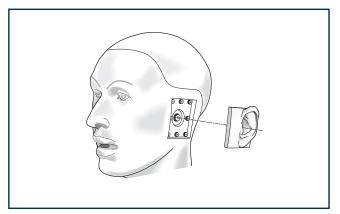
Most pinnae are push-mounted on eight studs. Anthropometric pinnae are secured with two screws
