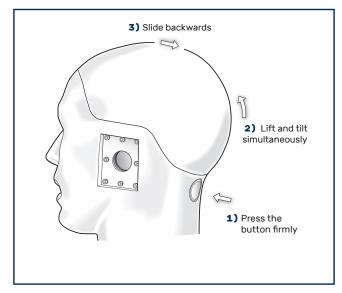
The top of the head is released by the push of a button
