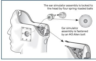
Ear simulators are easy to install and remove
