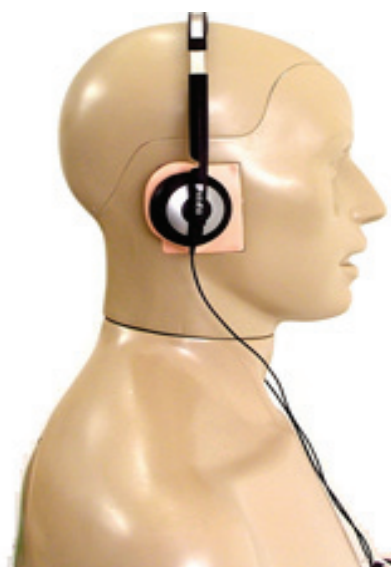
Fig. 2. 45BB Head and Torso simulator
