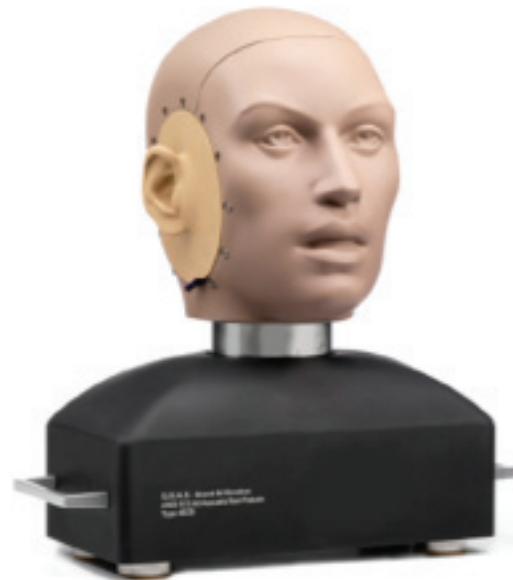
Fig. 10. Head and torso for high level hearing protector test
