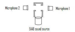
Figure 2: 51AB calibration - step 2 (Microphones have switched side compared to Fig. 1).
