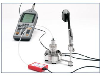
EAR 3A Ear-insert mounted on the IEC 60318-5 2cc Coupler. This setup is based on a 1" measurement microphone.
