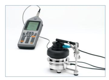
TDH-39 Supra-aural earphones mounted on the NBS 9-A / IEC 60318-3 6cc Coupler. This setup is based on a 1" measurement microphone.
