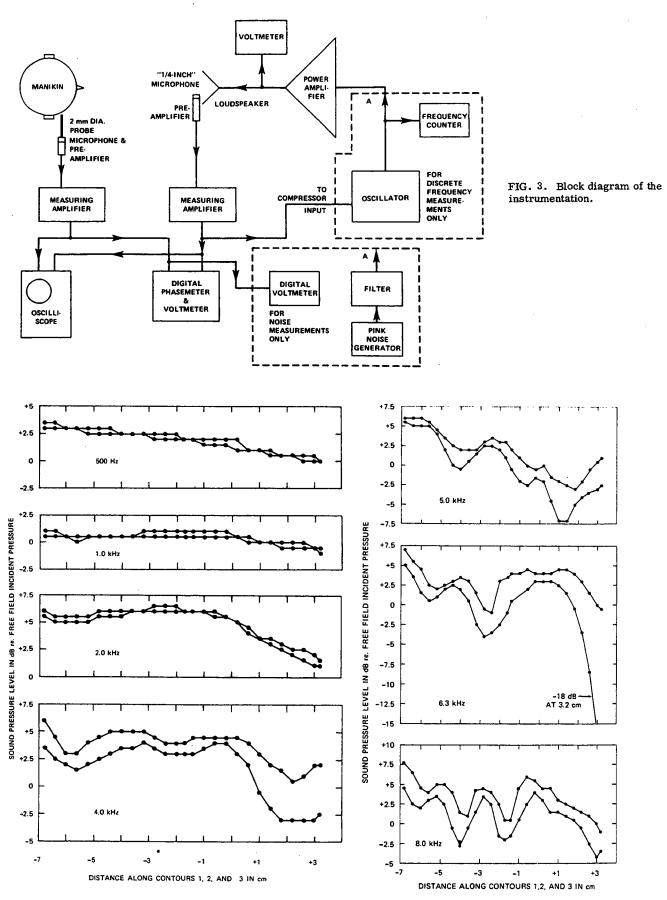
FIG. 4. Range of sound pressure levels for contours 1, 2, and 3 at 2, 4, and 7 mm from the head surface for discrete frequencies. Source-to-ear canal distance is 1.0 m.
