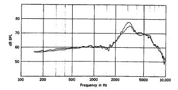
Fig. 8-2. The effects of KEMAR on a free sound field measured at the eardrum with source location at 0° azimuth for two test sessions eight days apart.
