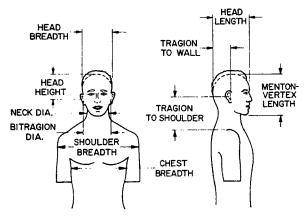
FIG. 1. Anthropometric measures used in design of KEMAR.
