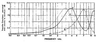
Fig. 15-8. Pressure ratio in ear canal (Shaw, 1974).
