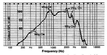
Fig. 9-14. Response at  $0^{\circ}$  incidence of a directional aid on KEMAR with and without wig.
