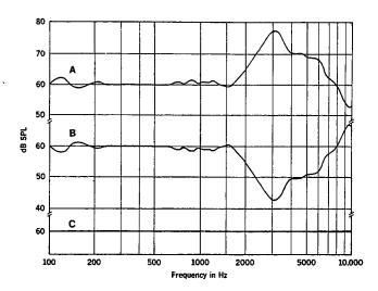
Fig. 8-3. Generation of the insertion gain test tape signal. Response A is KEMAR's response measured at the eardrum microphone to a constant input SPL signal at 0° azimuth. Response B is the sweep frequency test signal stored on magnetic tape. Response C is the sweep frequency signal measured at the eardrum microphone when response B, the test signal, is presented to KEMAR, response A.
