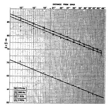
Fig. 9-3. Inverse square law measurements with single speaker.
