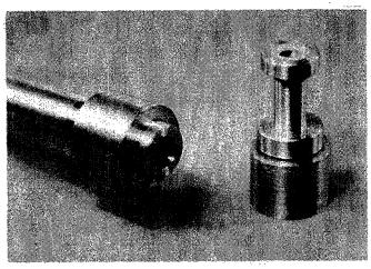
Fig. 16-5. An adapter for simulation of an earmold tube having internal dimensions of 18 mm length by 3 mm diameter. The adapter is shown with an XD-1053 two branch ear simulator.
