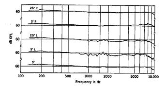
Fig. 8-6. Effects of slight azimuth angle changes on the insertion gain signal measured at KEMAR's eardrum microphone. After the initial insertion gain signal was generated, the manikin was rotated 2.5° and 5° left and right from 0° azimuth and then returned to the original 0° azimuth position.
