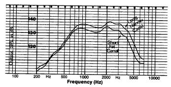
Fig. 9-15. Effect on SSPL90 of earmold canal length and O.D. using same bore diameter.
