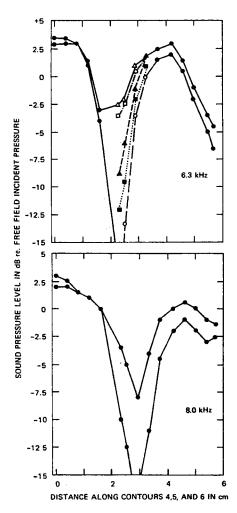
FIG. 7. Range of sound pressure levels for contours 4, 5, and 6 at 2, 4, and 7 mm from the head surface for discrete frequencies. Source-to-ear canal distance is 1.0 m. (At 6.3 kHz: open circles, 7 mm from head surface along contour 4; closed squares, 4 mm from head surface along contour 4; closed triangles, 2 and 4 mm from head surface along contours 4 and 5, respectively; open squares, 7 mm from head surface along contour 6; open triangles, 2 mm from head surface along contour 6.)
