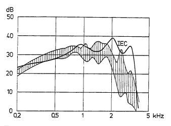
Fig. 5-3. Insertion gain for an over-the-ear hearing aid, frontal microphone location, on (5) five subjects and the gain measured by IEC methods.
