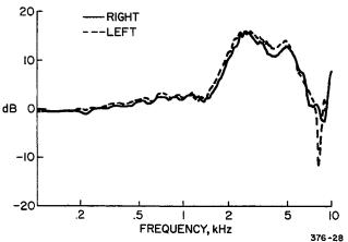
Fig. 10-7. Sound pressure at the eardrum in the KEMAR left and right ears for a free field sound pressure.
