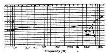
Fig. 9-13. Sound field at KEMAR eardrum with and without wig on KEMAR using tape recording for etymotic response made without wig.
