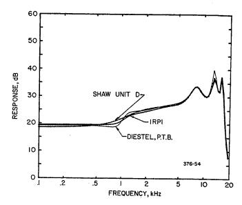
Fig. 15-13. Two branch occluded ear simulators: transfer impedance (multiplied by frequency) for a high impedance ceramic source. Computer calculated curves.
