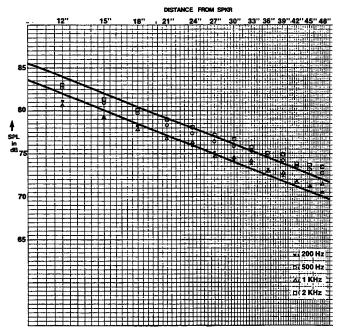
Fig. 9-2. Inverse square law measurements with 3 way speaker on 3 separate axes.
