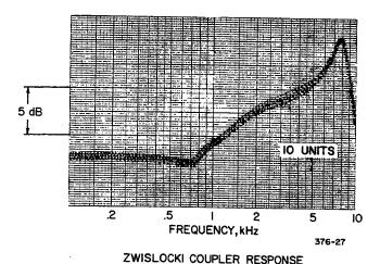
Fig. 15-5. The response of a high impedance experimental ceramic sound source on 10 Zwislocki type occluded ear simulators.
