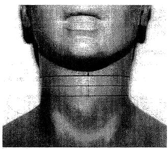
Fig. 3-4. The neck region of the KEMAR manikin showing marks applied for location of the head relative to the torso.
