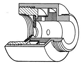
Fig. 15-9. Two branch ear simulator, type XD-1053.
