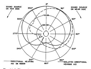
Fig. 11-2. The polar response at 2000 Hz for a directional hearing aid in a free field and mounted on the KEMAR manikin.
