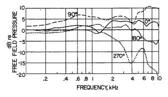
Fig. 3-9. Pressure on the surface of an earmold in the concha of a KEMAR ear when placed in a constant free field sound pressure.
