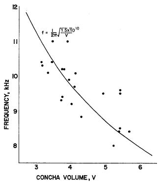
Fig. 3-2. The frequency of resonance,  $f_V$ , versus the volume,  $cm^3$ , of the concha for subjects used to investigate the acoustics of the external ear.
