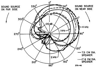
Fig. 10-9. Polar response of a directional hearing aid on the KEMAR manikin for three frequencies and for two different sized loudspeakers.
