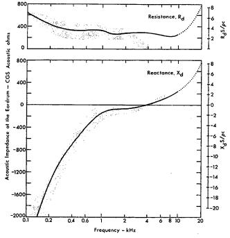
Fig. 15-7. Eardrum impedance design criteria (Shaw, 1974).
