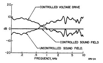
Fig. 10-2. The response curves showing servo controller operation to produce a constant sound field at the test point in a free field.
