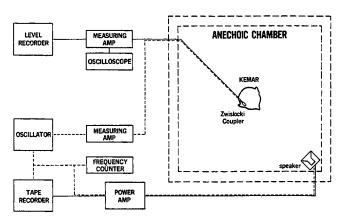
Fig. 8-1. Block diagram of the instrumentation used for measurement of hearing aids on KEMAR.
