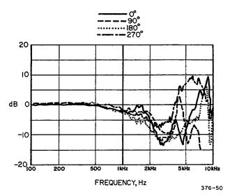
Fig. 12-8. Function to convert a pressure gain response of a hearing aid measured in a sound box with a Zwislocki coupler into an etymotic or insertion gain. The hearing aid is an over-the-ear, top microphone type.
