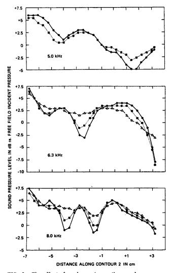
FIG. 9. The effect of random noise on the sound pressure level along contour 2 at 4 mm from the head surface; closed circles, tone; closed squares, 6% bandwidth pink noise; open triangles, 29% bandwidth pink noise. Source-to-ear canal distance is 1.0 m.
