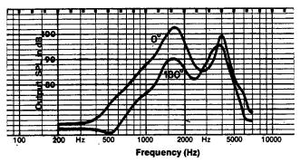
Fig. 9-11 (b). Directional ITE aid response on KEMAR using tape recorder to provide flat SPL at KEMAR eardrum with no aid present. Separate correction curves for 0°, 180° incidence.
