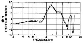
FIG. 11. Eardrum sound pressure in KEMAR showing effect of neck length on torso reflections.  $\cdots$  18.8 cm; ——17.6 cm; — - 16.3 cm.
