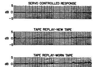
Fig. 10-3. Uniformity of first and twentieth tape play back sound field level compared to the level when the servo control is working directly.
