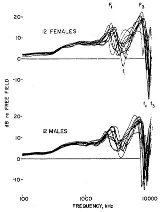
FIG. 4. Ear canal entrance sound pressures, 12 males, 12 females, sound source at 90° azimuth angle, 1m. Free field is the reference pressure condition.
