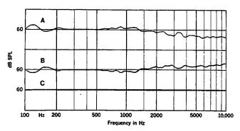
Fig. 8-5. Generation of the substitution taped signal. Response A represents the loudspeaker's response. Response B represents the sweep frequency test signal stored on magnetic tape. Response C is the sweep frequency signal measured at the test point when response B, the test signal, is presented through the loudspeaker, response A.
