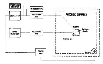
Fig. 8-4. Block diagram of instrumentation used for the two Zwislocki coupler measurements procedure on KE-MAR.
