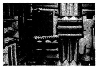
Fig. 9-1. Picture of KEMAR in anechoic chamber used for this study.
