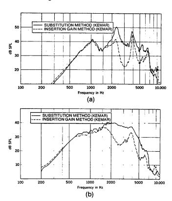
Fig. 8-7. Frequency responses of two hearing aids with the insertion gain and substitution measurement methods. The solid line is the substitution response and the dotted line is the insertion gain response.
