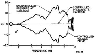
Fig. 11-4. The signals involved in producing a constant sound pressure as a function of frequency at the eardrum of the KEMAR manikin in an anechoic room. The manikin is 1 meter distant from an 8" loudspeaker.
