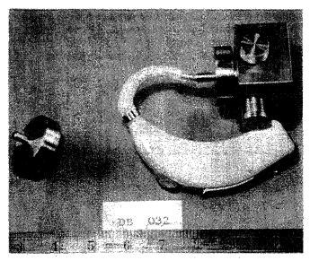
Fig. 16-3. Adapter for occluded ear simulator to connect to hearing aid tubing. The hole in the adapter would be equal to the inner-diameter of the tubing. The ear simulator shown is a Zwislocki four branch type.
