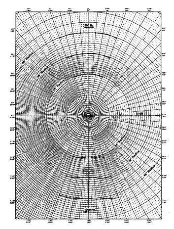
Fig. 9-4. Deviation from constant SPL, off speaker axis, on 3 radial lines in anechoic chamber at 500 Hz, 1 kHz.
