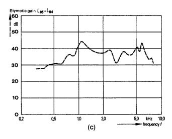
Fig. 6-3. Frequency response of a wide-range behind-the-ear hearing aid (Type C, cf. Fig. 6-6). Input Level L  $_1$  60 dB SPL, position of gain control to give 40 dB gain at 1 kHz under standard condition. (a) Output level L  $_{01}$  measured according to Standard condition IEC 118, IEC 126 (2 cm $^3$  coupler) (b) Output level L  $_{03}$  measured with the hearing aid on KEMAR (c) Calculated value L  $_{03}$ -L  $_{04}$  for etymotic gain.
