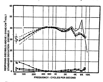
Fig. 13-2. Response of a Permoflux type PDR-8 dynamic earphone in an MX41/AR cushion measured by probe tube on persons. (Burkhard and Corliss (1954) ). The average response for the subjects as shown with the root variances of the mean  $S_{\text{o}},$  of measurements among people  $S_{\text{p}},$  between the two ears of a person  $S_{\text{e}},$  and for measurement error  $S_{\text{e}}$
