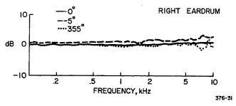
Fig. 10-6. The change in sound pressure at the right eardrum of the KEMAR manikin for small misalignments in the orientation of the manikin in a free sound field. Five degrees would cause the ear to be closer to the loudspeaker. 355° would cause the ear to be away from the loudspeaker in the shadow of the head.
