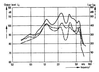
Fig. 6-7. Frequency response of a hearing aid with Type D Microphone Location. (microphone near hook through lower side of case). The code for the various curves is the same as in Fig. 6-3. Input level,  $L_{\rm I}=60$  dB SPL, position of gain control to give 40 dB gain at 1 kHz under standard conditions.
