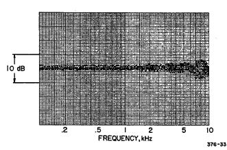
Fig. 10-4. A plot of the uniformity of the sound field on a 15.2 centimeter diameter circle, centered 93 centimeters from the source, for a constant free field pressure level at the center point of the circle.
