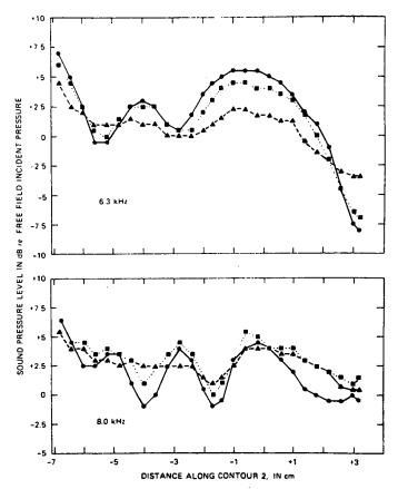
FIG. 14. The effect of random noise on the sound pressure level along contour 2 at 4 mm from the head surface for a source placed 3.5 m from the ear canal in front of the manikin: closed circles, tone; closed squares, 6% bandwidth pink noise; closed triangles, 29% bandwidth pink noise.
