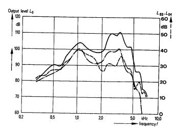
Fig. 6-5. Frequency response of a hearing aid with Type B Microphone Location. (microphone at the bottom of the case). The code for the various curves is the same as in Fig. 6-3. Input level,  $L_{\parallel}=60$  dB SPL, position of gain control to give 40 dB gain at 1 kHz under standard conditions.
