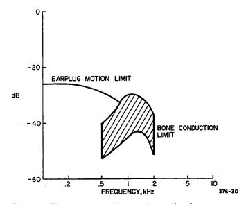
Fig. 13-5. Theoretical maximum attenuation for ear protectors according to Zwislocki.
