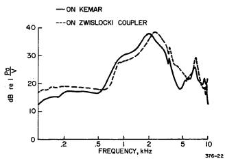
Fig. 13-3. Response of a Sharpe HA-10A circumaural earphone on a Zwislocki coupler and on the KEMAR.
