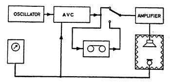
Fig. 10-1. A block diagram of the system for generating a tape recorded control signal for a constant free field.
