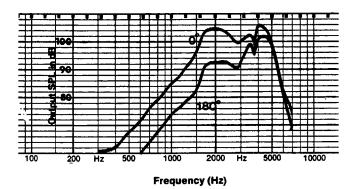
Fig. 9-10 (b). Directional ITE aid response on KEMAR using control microphone positioned on axis ½ way between KEMAR and speaker—input SPL 6 dB higher.
