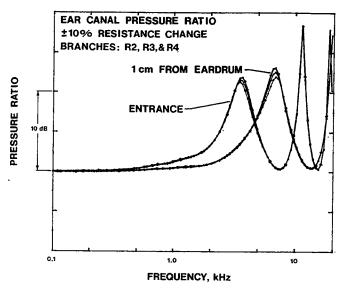
Fig. 15-3. Ear canal pressure ratio for a Zwislocki four branch type ear simulator, calculated from a computer model. The effect of resistance change in the branches is given also.
