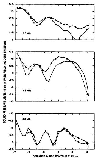
FIG. 13. Comparison of sound pressure level along contour 2 at 4 mm from the head surface for a source placed 1.0 and 3.5 m from the ear canal in front of the manikin; open circles, data for source-to-ear canal distance of 1.0 m; open triangles, data for source-to-ear canal distance of 3.5 m.
