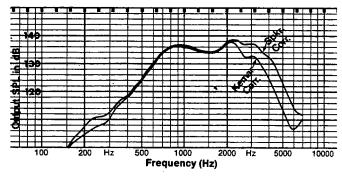
Fig. 9-9. SSPL 90 with substitution method (speaker correction) and etymotic method (KEMAR correction) inputs.
