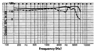
Fig. 9-12. Response at KEMAR eardrum with KEMAR at 180° incidence using tape recordings for flat SPL at eardrum at 0° incidence (-----) and at 180° incidence (
