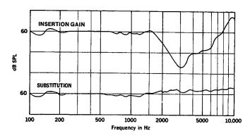
Fig. 8-8. Sweep frequency test signals for the insertion gain and substitution measurement methods.
