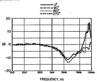
Fig. 12-7. Function to convert a pressure gain measured in a sound box with a Zwislocki type ear simulator into an etymotic or insertion gain. This is for an in-the-ear hearing aid with an occluded ear fitting.
