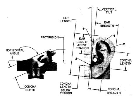
FIG. 3. Auricle measures used in design of KEMAR. (1) Upper pinnaskull notch; (2) antihelix; (3) intertragal notch; (4) crus of helix.
