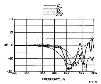
Fig. 12-9. Function to convert a pressure gain of a hearing aid measured in a sound box with a Zwislocki ear simulator into an etymotic or insertion gain. This is a behind-the-ear hearing aid with bottom microphone.
