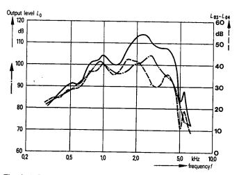
Fig. 6-4. Frequency response of a hearing aid with Type A Microphone Location. (frontal microphone through the hook). The code for the various curves is the same as in Fig. 6-3. Input level,  $L_{\parallel}=60$  dB SPL, position of gain control to give 40 dB gain at 1 kHz under standard conditions.
