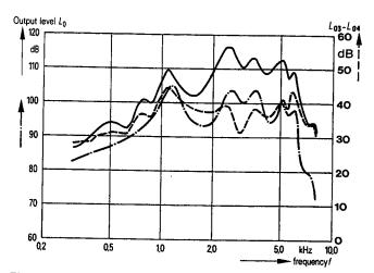
Fig. 6-6. Frequency response of a hearing aid with Type C Microphone Location. (microphone in frontal region through upper side of case). The code for the various curves is the same as in Fig. 6-3. Input level,  $L_1 = 60 \text{ dB}$  SPL, position of gain control to give 40 dB gain at 1 kHz under standard conditions.
