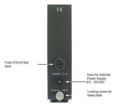
Fig. 2.3 Rear panel of the Power Module Type 12HF
