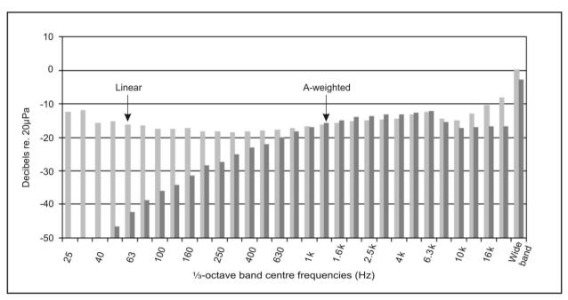
Fig. 1.6 Typical noise floor of Type 40HF for system and microphone. Shown in  $\frac{1}{3}$ -octave bands for both the linear and A-weighted cases
