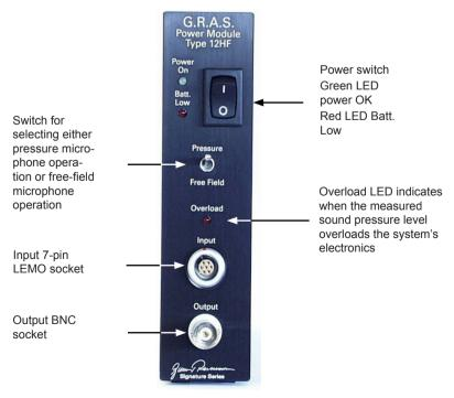
Fig. 2.1 Front panel of the Power Module Type 12HF
