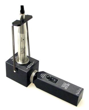
Fig. 3.2 Pistonphone fitted with Coupler RA0090 and the microphone inserted into the Coupler
