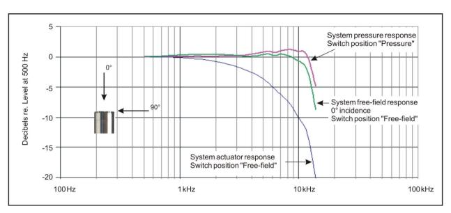
Fig. 1.4 Typical frequency response curves of Type 40HF
