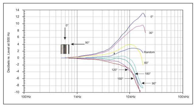
Fig. 1.5 Free-field corrections for various angles of incidence on the 1-inch Microphone Type 40EH.
