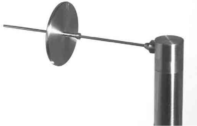
Fig. 2.8 Showing the Heat Sink GR0267 mounted on a stainless-steel probe
